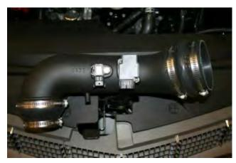
11. Transfer the air sensors from the Factory air box lid into the Airaid intake tube(#2). Do not use factory hardware! Secure the MAF sensor using the two #8-32x 1/2 screws (#16) and Lock Washers (#17), and the MAP sensor with the 1/4-20x3/4 bolt (#19). Install the Reducer Coupler and one #64 clamp(#26) and the #48 (#27) clamp on the 90 deg bend of the Intake Tube. Install the Hump Hose (#9) and 2 #64 clamps(#26) on the opposite end of the Intake Tube.
