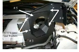
**6.** Install the Adapter Panel (#5) to the MAF Panel (#3) as shown using four 6-32 screws (#12), 6-32 Kep nuts, and #6 flat washers (#14). Attach the Rear Panel (#4) to the MAF Panel using two 6-32 screws.
