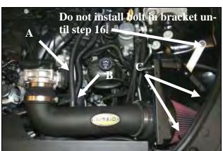
**15. A)** Replace the factory breather line on the valve cover with the 26" Airaid Breather Hose(#12). **B**) Secure the breather hose to the intake tube nipple using the black Speed Clamp (#32).C) Slide the Edge Clip Cable Ties (#31) about 6" apart along the fender pinch weld and return the coolant line to it's original location. Secure the coolant line using the cable ties and trim off
