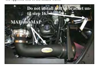
14. Install the Airaid Intake Tube assembly onto the filter adapter first, and then onto the throttle body. Adjust for fit, and tighten all the hose clamps. Next, reconnect the MAF and MAP sensors.
