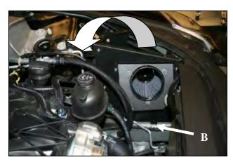
13. A) Lower the Airaid Performance Air box assembly into the engine cavity. Insert the Well Nut into the Factory core support grommet and rotate the assembly rearward until the bracket rests on the shock tower and the MAF panel's lower tab hole is lined up with the Tapped Chassis bolt hole from step 5. B) Secure the assembly by using the 1/4-20x 3/4 Bolt(#19).
