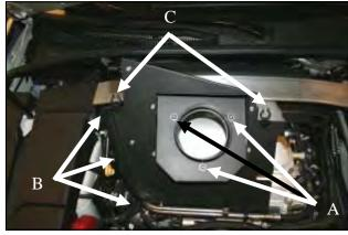
**9A)** Install the Filter Adapter onto the MAF panel using three 1/4-20 Button Head screws (#18) and 1/4" Flat washers (#17). **B)** Attach the Weather Strip (# 11) to the curved edge of the MAF Panel. **C)** Insert the 5/8" hose anchors (#30) into the two horizontal tab holes on the MAF panel.
