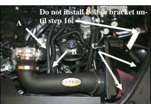
**15. A)** Replace the factory breather line on the valve cover with the 26" Airaid Breather Hose(#12). **B**) Secure the breather hose to the intake tube nipple using the black Speed Clamp (#32).C) Slide the Edge Clip Cable Ties (#31) about 6" apart along the fender pinch weld and return the coolant line to it's original location. Secure the coolant line using the cable ties and trim off
