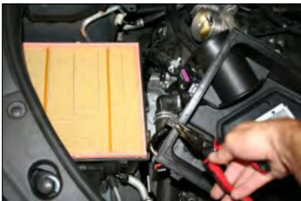
4. Turn the factory airbox lid over and locate the wire harness anchor. Using a pair of needle nose pliers, compress the ribs of the anchor and remove it. Remove the factory air filter and set it aside.
