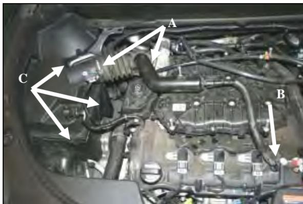
2. A) Loosen the hose clamps on the factory intake tube. B) Disconnect the crank case breather line at the valve cover, and remove the factory intake tube. C) Unfasten the 3 Factory air box clips.
