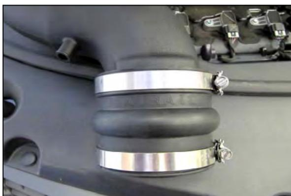
8. Place a #52 Hose Clamp (#18) onto each end of the Hump Hose (#6), and slide onto the Throttle body side of the Intake Tube as shown. Do not tighten the clamps at this time.
