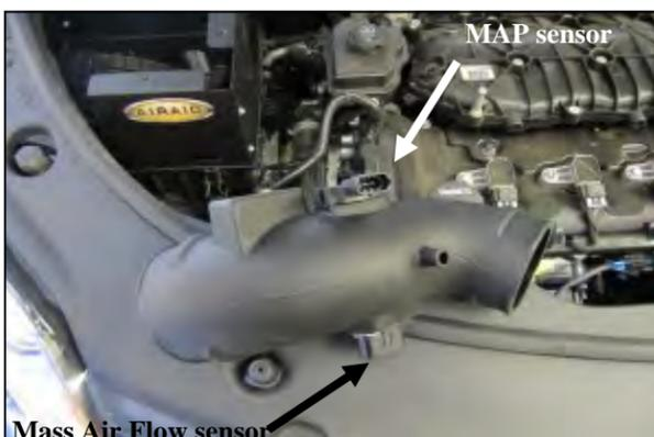
7. Transfer the air sensors from the factory airbox lid into the Airaid Intake Tube(#2) as shown. **Do Not Use The Factory Hardware.** Secure the Mass Air Flow sensor using the two #8-32 screws (#16), and the MAP sensor using the 1/4-20x 3/4 hex head bolt (#9) and 1/4" Flat Washer (#12).
