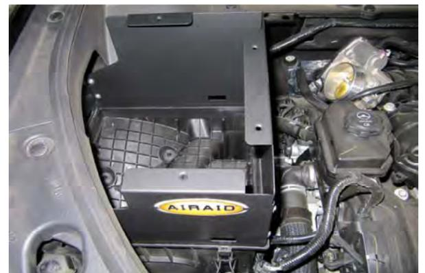
6. Slip the Airaid Panel tabs into the slots in the factory airbox and partially install the Panel assembly onto lower half of the factory airbox as shown. Do not latch the airbox clips at this time.
