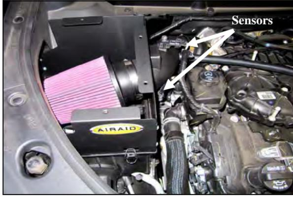
**12.** Install the Airaid Premium Filter (#1) to the Intake Tube. Reconnect the Mass Air Flow and MAP sensors.
