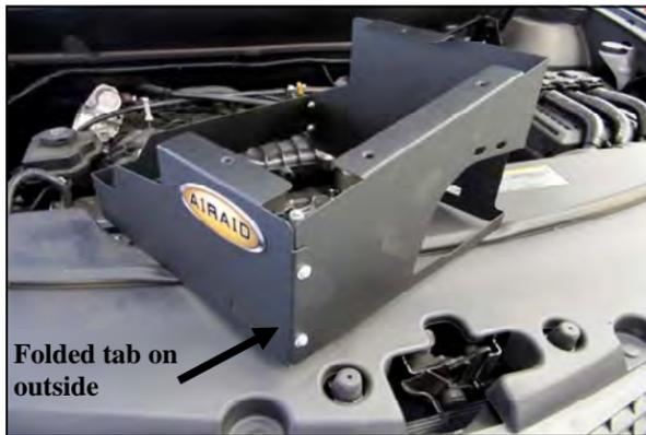
5. Join the two Airaid panels together with the folded tabs on the **outside**, using the four 6-32 screws (#15), #6 Flat washers (#14), and #6 Keps Nuts (#13).
