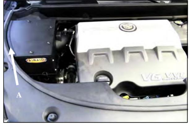
**13.** **A)** Attach the Weather Strip (#7) to the curved edge of the Top Panel (#5). **B)** Attach the Top Panel to the Airaid Performance Airbox using the four 1/4-20 Phillips Head Screws. Reinstall the engine cover and the oil fill cap.
