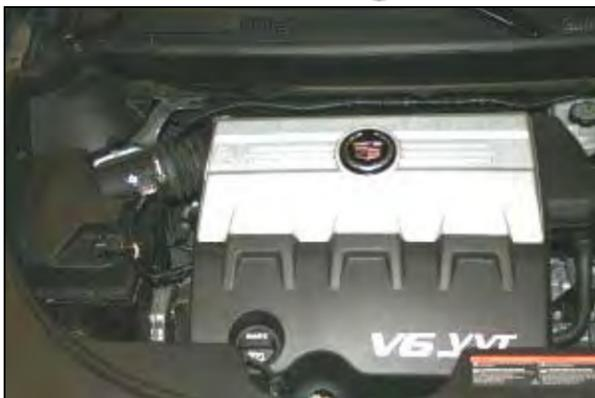
1. **Disconnect the negative battery cable.** Remove the oil fill cap and then lift up on the front of the engine cover to remove it from the vehicle. Replace the oil cap for now to make sure nothing falls into the valve cover during the install.
