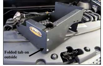
5. Join the two Airaid panels together with the folded tabs on the outside, using the four 6-32 screws (#15), #6 Flat washers (#14), and #6 Keps Nuts (#13).
