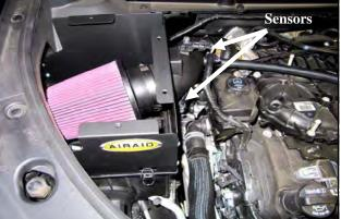
**12.** Install the Airaid Premium Filter (#1) to the Intake Tube. Reconnect the **M**ass **Air F**low and **MAP** sensors.
