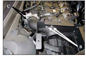
9. A) Insert the Filter end of the Intake Tube into the Panel assembly opening and guide the Coupler side onto the throttle body. **B**) Rotate the Intake Tube until the mounting holes are aligned with the Panel holes. Secure the Intake Tube to the panel assembly using the two 8-32 button head screws (#16). C) Tighten the Hose Clamps, and fasten the airbox clips at this time.
