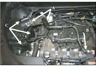
2. A) Loosen the hose clamps on the factory intake tube. **B**) Disconnect the crank case breather line at the valve cover, and remove the factory intake tube. C) Unfasten the 3 Factory air box clips.
