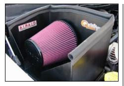
**11.** Mount the Airaid Premium filter inside the Cool Air Dam & secure with hose clamp provided. In addition, install the weather strip hood seal on the Cool Air Dam. (<u>Hint</u>: begin in a corner and work it on toward the ends)
