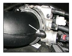
**16.** 2004 Models Only: Slide the provided rubber cap over the nipple at the throttle body end of the Airaid tube.
