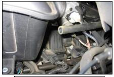
5. 2002 & 2003 Models Only: Disconnect the crankcase vent hose on the back of the factory throttle body air chamber.
