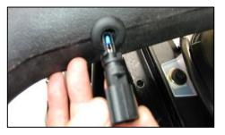
9. 2003 & 2004 Models Only: Install rubber grommet w/<u>thru</u> <u>hole</u> and insert the factory air temperature sensor into the grommet.
