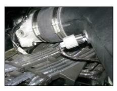
**14.** Re-connect air temperature sensor connector to the sensor in the Airaid tube.
