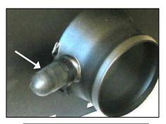
17. 2002 & 2003 Models Only: Slip the black rubber cap over the nipple on the Cool Air Dam and secure using the #19 Snapper clamp provided.
