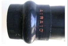
12. Install black hump hose onto the Airaid tube and secure using a # 60 hose clamp provided.
