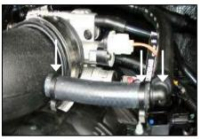
15. 2002 & 2003 Models Only: Use the 90° plastic elbow provided, connect the factory breather hose with the 4 <sup>1</sup>/<sub>2</sub>" hose to the Airaid tube & secure using the three #16 black Speed clamps.
