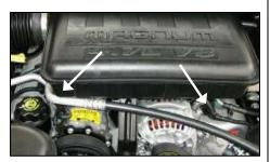
4. Loosen and remove the two 10mm bolts holding on the factory throttle body air chamber intake assembly.
