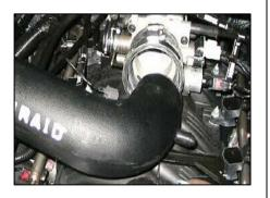
**13.** Position Airaid tube into place by connecting hump hose to Airaid Cool Air Dam and connect the other end of the tube to the factory throttle body coupler. Utilize the #60 hose clamps on the hump hose and #56 hose clamp on the factory coupler.
