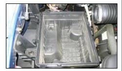
**3.** Unsnap and remove the factory air box lid, tube, & factory air filter.
