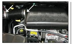
1. Disconnect the negative battery cable and loosen the two hose clamps on the factory air tube
