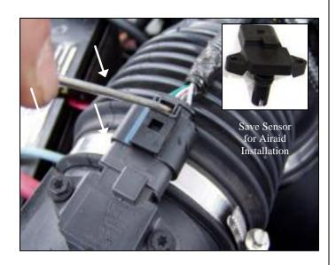
1. Disconnect the negative battery cable and disconnect the electrical connector. Using the T-20 bit loosen the two star head bolts and remove the electrical sensor. (Retain sensor for installation of Airaid Intake System)
