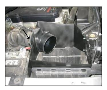
6. Install Airaid intake assembly in place of the factory air box lid & tighten factory hose clamp on intake tube to Airaid system & secure air intake tube to adapter using the factory hose clamp.
