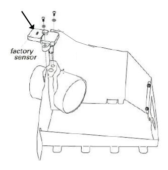
**5.** Fasten the factory sensor on top of the adapter using the (2) 8/32 screws and washers using a 3/32 Allen Wrench.
