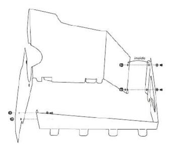
**3.** Assemble Airaid Quick Fit Cold Air Dam panels using the (4) 6/32 screws, washers and nuts provided.
