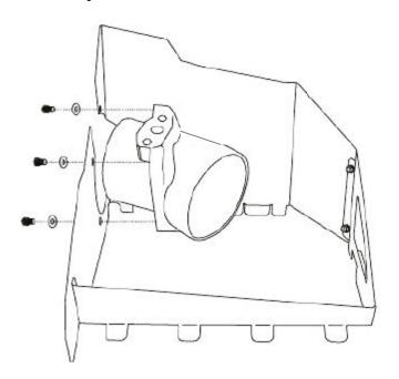
**4.** Assemble the air filter adapter to the cold air dam using the (3) ½-20 bolts and washers provided.
