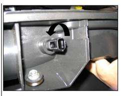
**7.** Remove air temperature sensor from housing by turning counter clockwise and pull.
