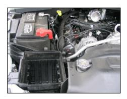
**3.** Remove lid from air box base. Using a 13mm socket, remove air box base from engine compartment.
