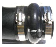
13. Install the hump hose and coupler provided onto the Airaid MIT with the supplied hose clamps. The straight coupler is positioned on the throttle body end and the hump hose is positioned on the air filter end.
