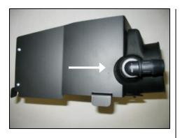
**10.** Install the supplied nylon fitting into the air filter adapter as shown.
