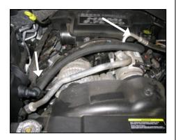
11. Remove factory breather hose. Using the supplied straight ¾" hose, connect both ends to the nylon fitting and oil fill nipple as shown. Fasten both ends using the supplied nylon speed clamps. Adjust the nylon fitting downward to clear the Airaid intake tube assembly.
