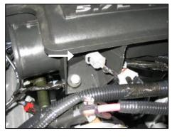
**5.** Carefully disconnect electrical connector from air temperature sensor in factory housing.
