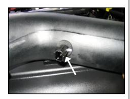
**12.** Install the supplied grommet and factory air temperature sensor into the Airaid Modular Intake Tube.
