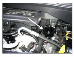
**6.** Remove oil fill cap from valve cover. Using 10mm socket, loosen two factory housing bolts. Remove housing from engine. Replace oil fill cap.
