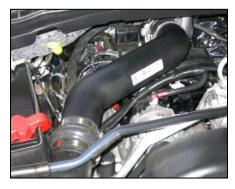
**14.** Check for any foreign objects or debris it the intake path & install Airaid MIT assembly on engine. (*Note: Leave hose clamps loose until final assembly*)
