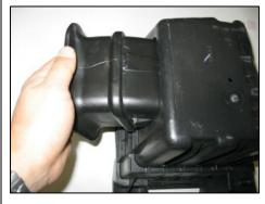
4. Using a flat blade screwdriver, carefully unsnap the box inlet from the base and remove it. Reinstall the factory base in the engine compartment with out the inlet.
