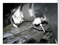
**15.** Reconnect electrical connector on factory air temperature sensor.
