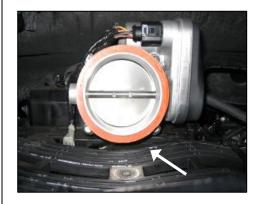
**8.** Remove factory orange seal from throttle body.
