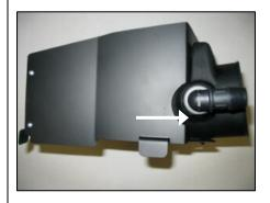
**9.** Install the supplied nylon fitting into the air filter adapter as shown.
