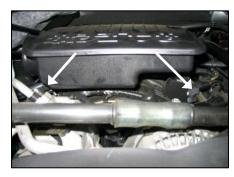
**6.** Loosen the two 10mm bolts mounting the factory air box to the intake manifold and remove from vehicle.
