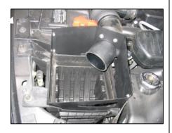
**10.** Install the Airaid Quick Fit assembly on top of the factory air filter base. Relatch the clips, and tighten the hose clamp.
