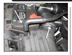
1. Disconnect the negative battery cable. Disconnect the breather hose from the factory air box lid. Loosen the two hose clamps on each end of the factory intake tube.
