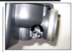
7. Turn the air temperature sensor \( \frac{1}{4} \) turn and remove from the air box. Retain sensor for later use.
