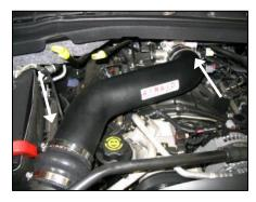
**14.** Install the Airaid intake tube assembly by connecting the Airaid hump hose onto the air filter adapter, and the other end into the Airaid reducing coupler. Tighten all hose clamps.
