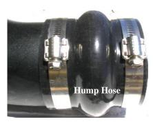
**13.** Slide the hump hose on to the straight end of Airaid intake tube with two #56 hose clamps. (*Note: Leave hose clamps loose until final assembly*).
