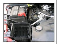
3. Unlatch the metal clips and remove the lid from air box base. Using a 13mm socket, remove the air box base from the engine compartment.
