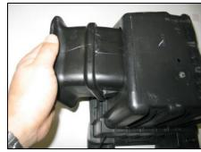
4. Using a flat blade screwdriver, carefully unsnap the box inlet from the base and remove it.
