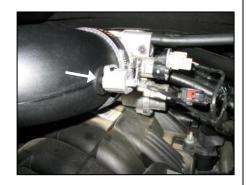
15. Install the supplied rubber grommet and factory air temperature sensor into the Airaid intake tube. Next, reconnect the factory electrical connector onto the sensor.
