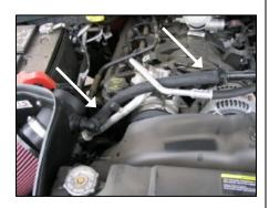
11. Using the supplied pre-formed 3/4" breather hose, connect the nylon fitting to the remaining plastic factory hose as shown. Fasten both ends of the hose using the supplied nylon speed clamps. Adjust the fitting downward to clear the factory intake tube assembly.
