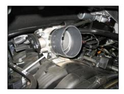
**12.** Install the supplied reducing coupler and #52 hose clamp onto the throttle body.
