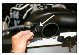
9. Carefully install the air temp sensor into the grommet in the Airaid Intake Tube. Make sure it goes all the way in.
