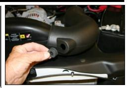
7. Install the supplied grommet into the Airaid Intake Tube.
