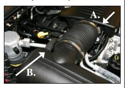
2. A.) Loosen hose clamp on the resonator end of intake tube.B.) Disconnect breather hose from factory airbox.
