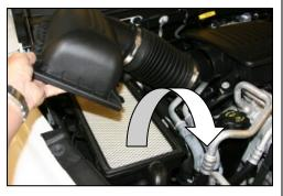
**3.** Remove the top of the factory airbox, and tube. Remove the factory air filter.
