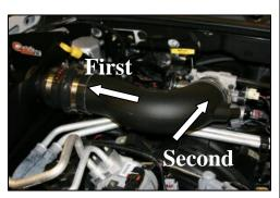
**11.** Slide the Airaid Intake Tube into the hump hose first, and then into the reducer on the throttle body. Adjust the tube for fit, and tighten the clamps.
