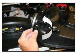
**8.** Carefully twist and remove the air temp sensor from the factory resonator.
