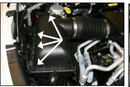
**1. Disconnect the negative battery cable.** Unlatch the 4 clips on factory airbox.
