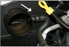
6. Reconnect the breather hose to the Quick Fit Panel and install the speed clamp as shown.
