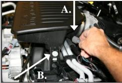
4. A.) Disconnect the air temperature sensor. B.) Remove 2 bolts (one on each side) that hold the resonator to the intake manifold and remove the resonator.
