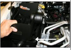
5. Install the Quick Fit Panel onto the top of the factory airbox. Slip the five tabs thru the slots on the airbox, adjust the panel on top and re-snap 2 of the latches.
