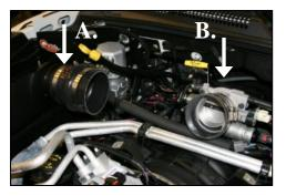
**10.** A.) Install the hump hose on the Quick fit Panel. (Leave clamps loose.) B.) Install the reducing coupler on the throttle body. (Leave clamps loose.)
