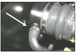
**15.** Slip the #24 speed clamp (#11) over the factory breather hose and re-connect the factory breather hose to the nipple on the CAD. Squeeze the clamp to retain the hose in place.
