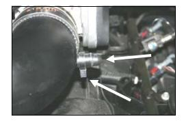
**12.** Install the provided rubber cap (#7) and speed clamp (#10) onto the nipple on the Modular Intake Tube, as shown.
