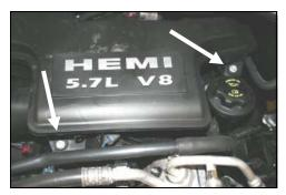
**4.** With a 10mm socket, remove two bolts holding the intake resonator to the intake manifold. Lift and pull resonator away from the throttle body and remove it from the vehicle.
