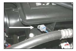
**3.** Squeeze the tab on the connector, and disconnect the intake temperature sensor.
