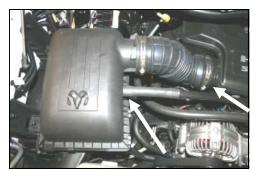
1. **Disconnect the negative battery cable!** Loosen the hose clamp on the resonator. Disconnect the breather hose going into the fac-
