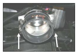
**10.** Install the reducing coupler (#5), small end first, onto the throttle body using two #52 hose clamps (#8). Leave clamps loose.
