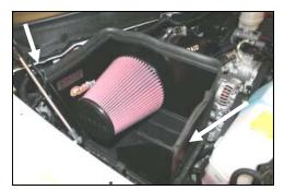
**14.** Install the Airaid Premium Filter (#1) onto the tube on the CAD and tighten the clamp. Next install the weather strip (#6) on the top of the CAD as shown. (*Hint: Start at one end of the CAD and work your way towards the other end.*)
