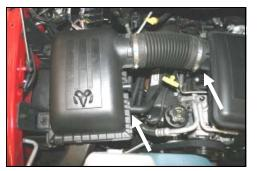
1. **Disconnect the negative battery cable!** Loosen the hose clamp on the resonator. Disconnect the breather hose going into the factory airbox lid.
