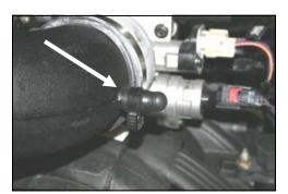
**14.** Install the provided rubber cap (#10), and speed clamp (#7) onto the nipple on the Modular Intake Tube (#3).
