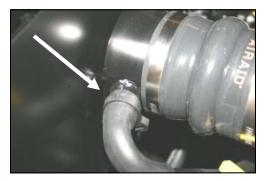
**12.** Install the provided #24 speed clamp (#8) over the factory breather hose, then slide the hose onto the nipple on the CAD. Squeeze the clamp to secure the hose.
