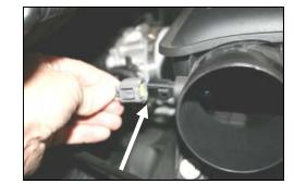
**3.** Squeeze the tab on the connector, and disconnect the air intake temperature sensor on the back of the resonator.
