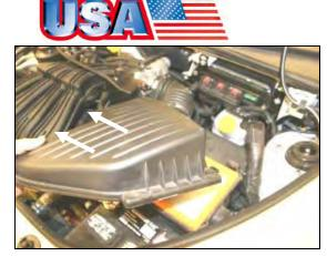
**3.** Remove the factory air cleaner lid by lifting up on the front, and then sliding the tabs out of the back of the air cleaner base.
