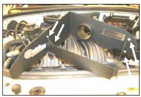
**7.** Assemble the Quick Fit Panels (#2 & #3) as shown, using the four provided screws (#8), washers (#9), and nuts (#10).
