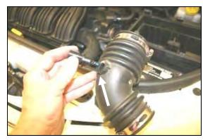
**6.** Carefully remove the temperature sensor from the factory intake tube and set it aside, it will be reused in step #10.
