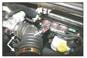
1. **Disconnect the negative battery cable.**Slide the red tab up on the temperature sensor, and then squeeze the black tab at the top of the sensor, and disconnect the wiring harness from the temperature sensor. Next loosen the two hose clamps at each end of the factory intake tube.
