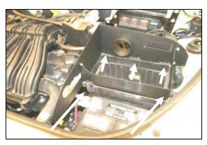
**8.** Install the three tabs of the assembled Quick Fit Panel into the three slots on the back of the factory air cleaner base, adjust the panels to fit in the slot around the top of the base, and re-latch the two factory clips to secure the panels to the base.
