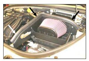
12. Install the Airaid Premium Filter (#1) onto the Quick Fit Panel, and tighten the hose clamp. Next install the weather strip (#6), as shown, onto the top of the Quick Fit Panel starting at the front and working your way towards the back.
