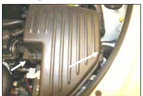
**2.** Unhook the two metal clips that hold the factory air cleaner lid to the base of the air cleaner box.
