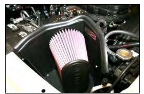
**15.** Install the Airaid Premium Filter (#1) onto the Airaid filter adapter, and tighten the hose clamp. Install the weather strip (#7) onto the top of the **CAD**, starting at the fender, and working your way towards the radiator.
