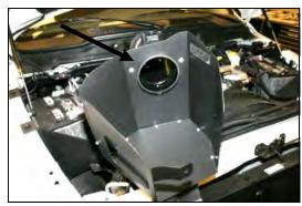
**10.** Assemble the Cool Air **D**am panels as shown using the seven 6-32x5/16" screws (#8), #6 flat washers (#9), and keps nuts (#10). Next install the Airaid filter adapter thru the **CAD** panel using three 1/4-20x1/2" button head bolts (#11), and 1/4" flat washers (#12). (See Arrow)
