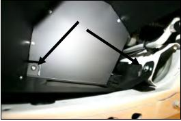
11. Install the CAD assembly into the vehicle, and install the 3/8-16x1" button head bolt (#18) thru the panel, and into the well nut. Next install the 6x1x12mm hex bolt (#16), and 1/4" flat washer (#12), thru the panel, and into the captured nut in the radiator support. Leave all bolts loose until final adjustment.
