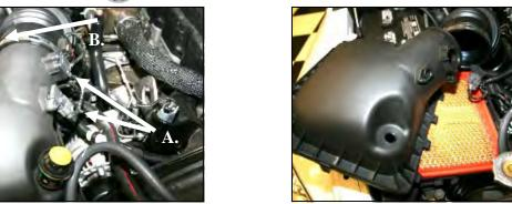
**2.** Unsnap the two metal clips that hold the airbox lid to the base, and remove the lid. Next, remove the factory paper air filter from the base.
