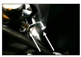
**12.** Using one 1/4-20x1/2" button head bolt (#11), 1/4" flat washer (#12), and 1/4" serrated nut (#13), and the 8x1.25x30mm hex bolt (#14), and 5/16" flat washer (#15), mount the supplied bracket (#19) between the **CAD** panel, and the fan shroud mounting boss as shown. Tighten all **CAD** mounting bolts at this time.
