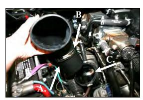
9. A) Install the metal tube (#5) into the rubber elbow (#6) until the rolled bead touches the side. B) Install one #80 hose clamp (#20) around the elbow at the metal tube, and tighten. C) Install the tube assembly into the factory rubber elbow on the turbocharger. Leave the factory hose clamp loose until final adjustments are made.
