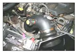
11. Install the Airaid Intake Tube (#2) into the factory turbo elbow and then into the hump hose. Adjust for fit, and then tighten all three hose clamps. Reinstall the factory grommet and filter minder, intake temperature sensor and Mass Air Flow sensor into the Airaid Intake Tube using three 8-32 button head screws (#7) and #8 flat washers (#8). **Do Not Use The Factory Screws!** Reinstall the factory wiring harness anchor into the hole in the Airaid Intake Tube.
