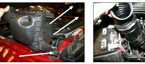
**3.** Loosen the hose clamp that secures the factory intake tube assembly to the rubber elbow on the turbo inlet, and remove the assembly from the vehicle.
