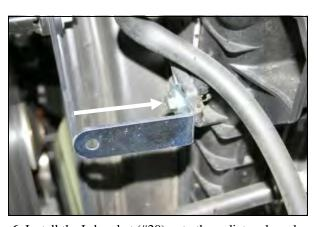
**6.** Install the L-bracket (#20) onto the radiator shroud as shown using one M8 x 30mm bolt (#14) and one flat washer (#12) as shown. Leave the bolt slightly loose for now.
