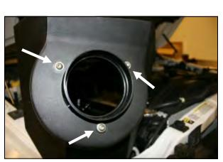
**8.** Install the filter adapter (#4) into the Cool Air Box (#3) using three 1/4" Button Head bolts (#9) and flat washers (#10) as shown.
