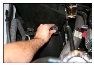
7. Install the Two supplied well nuts (#14) into the factory airbox mounting holes as shown.
