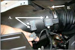
1. Disconnect the negative battery cables. A) Disconnect the air sensors on the upper half of the Factory Airbox, and detach the wire harness. B) Loosen the hose clamp that secures the factory intake tube assembly to the Airbox, unclip the Airbox lid, and remove the upper half of the factory airbox from the vehicle.
