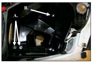
9. Install the CAB into the vehicle as shown. A.) Install the 3/8" button head bolts (#15) and flat washer (#16) thru the CAB and into the well nuts. B.) Install the 5/16" bolt (#11) flat washer (#12), and flange nut (#13) thru the CAB and L-bracket. Tighten all mounting bolts at this time.
