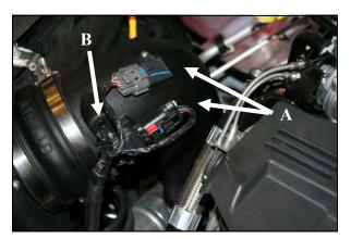
11. A) Install the Airaid Intake Tube (#2) into the factory turbo elbow and then into the hump hose. Adjust for fit, and then tighten all three hose clamps. Reinstall the intake temperature sensor and Mass Air Flow sensor into the Airaid Intake Tube using three 8-32 button head screws (#7) and #8 flat washers (#8). Do Not Use The Factory Screws! B) Reinstall the factory wiring harness anchor into the hole in the Airaid Intake Tube.
