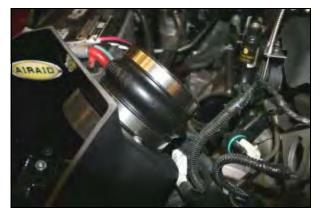
**10.** Install the supplied hump hose (#5) onto the filter adapter using two #72 hose clamps (#17). Leave the clamps loose for now.
