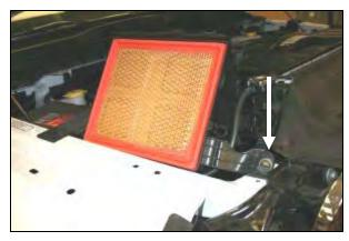
2. Using a 10 mm socket, remove the nut that secures the factory airbox, lower half, to the radiator support. Rock the factory airbox assembly side to side to release it from it's mounting grommets, and remove it from the vehicle.
