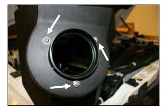
8. Install the filter adapter (#4) into the Cool Air Box, (CAB),(#3) using three 1/4" Button Head bolts (#9) and flat washers (#10) as shown.
