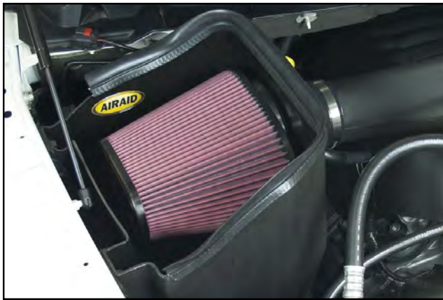
17. Install the Airaid Premium Filter onto the Filter Adapter inside the Cool Air Box. Install the Weatherstrip onto the Cool Air Box as shown, with the contour rolling away from the Filter.
