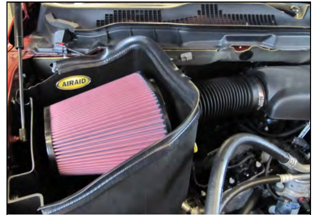
12. Install the Airaid Premium Filter onto the Filter Adapter inside the Cool Air Box. Install the Weatherstrip onto the Cool Air Box as shown, with the contour rolling away from the Filter.
