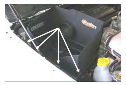
**3.** Position the Airaid Cool Air Dam (CAD) (#2) onto the factory airbox base. Relatch the factory clips onto the CAD.
