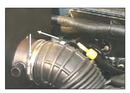
**4.** Reconnect the factory intake tube onto the **CAD**, and tighten the factory hose clamp.
