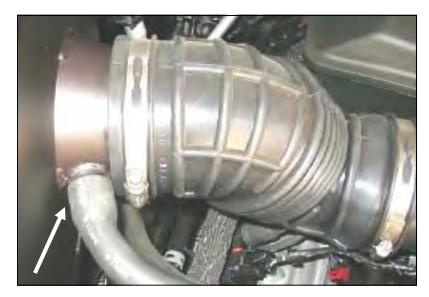
**6.** <u>2004-2005 Models Only</u>: Reconnect the factory breather hose to the nipple on the **CAD** and secure it using one #24 speed clamp (#4).
