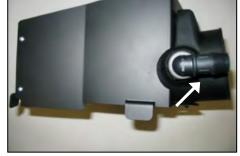
**5.** Install the supplied nylon fitting into the air filter adapter as shown.
