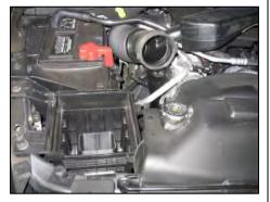
**2.** Loosen the hose clamp on the air box lid and remove the lid from the air box base.
