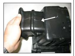
**3.** Using a 13mm socket, remove the air box base from the engine compartment. Using a flat blade screwdriver, carefully unsnap the box inlet from the base and remove it. Reinstall the factory base in the engine compartment without the inlet.
