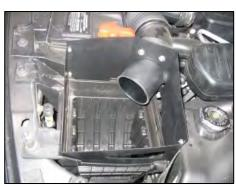
**6.** Install the Airaid Cool Air Dam assembly on top of the factory air filter base. Reconnect the factory intake tube, and tighten the hose clamp.
