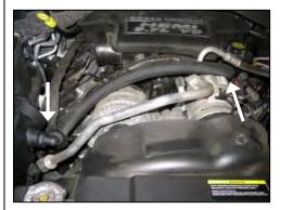
8. 5.7 Hemi engines only. Using the supplied straight <sup>3</sup>4" hose, connect both ends to the nylon fitting and oil fill nipple as shown. Fasten both ends using the supplied nylon speed clamps. Adjust the nylon fitting downward to clear the factory intake tube assembly.
