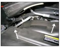
**7.** *4.7L engines only.* Using the supplied pre-formed 3/4" hose, connect the nylon fitting to the remaining plastic factory hose as shown. Fasten both ends of the hose using the supplied nylon speed clamps. Adjust the fitting downward to clear the factory intake tube assembly.
