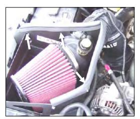
**15.** Install the Airaid Premium Filter (#1) onto the air filter adapter. Install the weather strip (#6) onto the top of the **CAD.** (Hint: start at one end, and work to the other).
