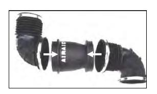
6. Replace the factory silencer tube with the Airaid Intake tube (#4). Complete the Airaid Intake tube assembly by aligning the notches in the tubes, and tightening the factory hose clamps.
