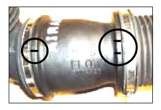
7. Note: Each side of the Airaid Intake Tube has notches that must be aligned with the notches on the factory intake tubes. Also, the flow arrow must point down toward the turbocharger inlet.
