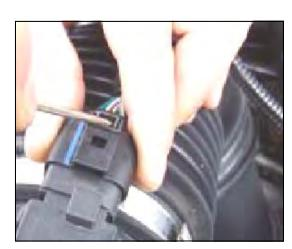
**14.** Reconnect the **MAF** sensor wiring harness to the sensor.
