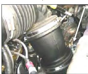
8. Install the Airaid Intake Tube assembly onto the turbocharger inlet. Tighten the factory hose clamp.
