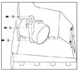
**10.** Mount the air filter adapter (#5) onto the **CAD**, using three 1/4-20x 5/8" hex bolts (#10), and three 1/4" flat washers (#11).
