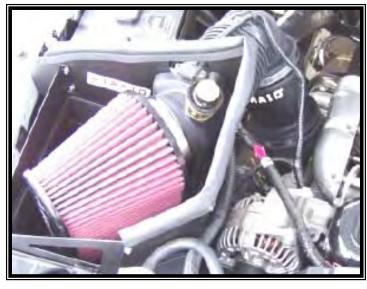
Synthamax Air Filters <u>do not</u> require <u>oil</u>. Service air filter as needed by cleaning with common non-petroleum all-purpose household cleaner and water. Simple Green®, Formula 409® or equivalent works great. Apply cleaner to outside of air filter and allow to soak. Then flush filter clean from the inside out with a garden hose and repeat steps if necessary. Do not apply high pressure water or air to clean filter. Allow filter to air dry and reinstall.
