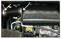
1. Disconnect the negative battery cable and loosen the two hose clamps on the factory air tube
