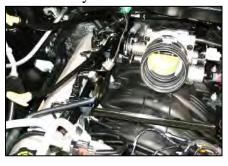
7. Unsnap the factory intake assembly from front of bracket and remove assembly from vehicle. (*Note: leave the factory coupler on the throttle body*)
