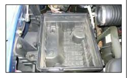
**3.** Unsnap and remove the factory air box lid, tube, & factory air filter.
