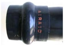
**12.** Install urethane hump hose onto the Airaid tube and secure using a # 60 hose clamp provided.
