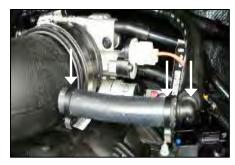
Use the 90° plastic elbow provided, connect the factory breather hose with the 4 ½" hose to the Airaid tube & secure using the three #16 black Speed clamps.
