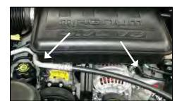
4. Loosen and remove the two 10mm bolts holding on the factory throttle body air chamber intake assembly.
