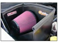
11. Mount the Airaid Premium filter inside the Cool Air Dam & secure with hose clamp provided. In addition, install the weather strip hood seal on the Cool Air Dam. (<u>Hint:</u> begin in a corner and work it on toward the ends)
