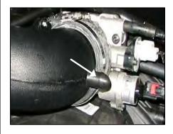
**16.** 2004-05 Models Only: Slide the provided rubber cap over the nipple at the throttle body end of the Airaid tube.
