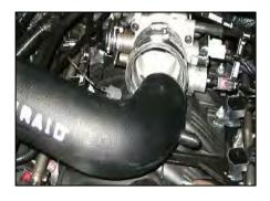
by connecting hump hose to Airaid Cool Air Dam and connect the other end of the tube to the factory throttle body coupler. Utilize the #60 hose clamps on the hump hose and #56 hose clamp on the factory coupler.
