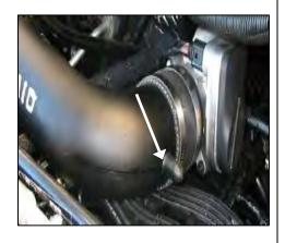
**18.** 2004-05 Models Only: Slide the black rubber cap over the nipple near the throttle body end of the Airaid Tube.
