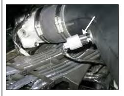
**16.** Re-connect air temperature sensor connector on the front of the tube.
