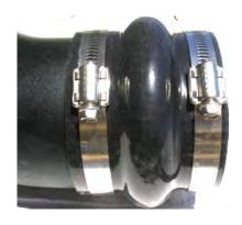
13. Install the urethane hump hose on the long end of the Airaid tube using two of the #60 hose clamps provided. Leave loose for final assembly.
