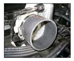
14. Slide the urethane coupler onto the throttle body and secure using a #60 hose clamp provided & install the 2<sup>nd</sup> #60 hose clamp on the other end of the coupler, leave loose for final assembly.
