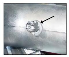
12. Install the rubber grommet into the hole on the front side of the Airaid tube & insert the factory air temp sensor into grommet.
