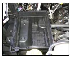
Unclip & remove the factory air box lid and factory air filter.
