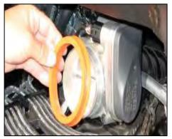
**6.** Remove the factory resonator and rubber seal from throttle body.
