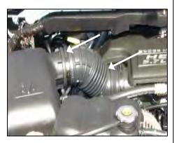
1. Disconnect the negative battery cable, and remove the factory "accordion" style intake hose by loosening the two factory clamps.
