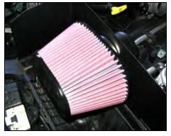
8. Mount the Airaid Premium filter inside the Cool Air Dam and secure with hose clamp provided.
