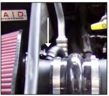
16. Reconnect the crankcase breather hose to the tube on the Airaid Cool Air Dam and secure with the black speed clamp provided. (*Note for* 2004: *Replace breather hose with new <sup>1</sup>/<sub>2</sub>*" *ID hose and speed clamps provided.*)
