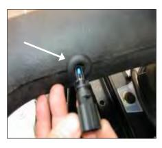
14. <u>If your vehicle is equipped</u> with an air temperature sensor, insert the rubber grommet into the hole on the intake tube and mount the air temperature sensor into the grommet.
