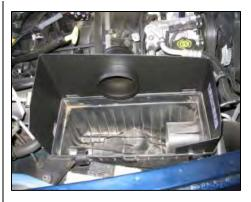
7. Mount the Airaid Cool Air Dam in place of the original air box lid & snap into place.
