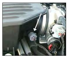
4. <u>If your vehicle is equipped</u> with an air temperature sensor, disconnect and remove the sensor & retain for later installation with Airaid kit.
