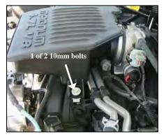
Loosen and remove the two 10mm bolts below the silencer box.
