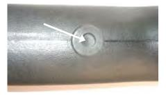
**15.** <u>If your vehicle is not equipped</u> with an air temperature sensor, insert the rubber grommet plug into the hole on the intake tube.
