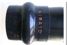
**10.** Install the urethane hump hose onto larger end of the Airaid Intake tube using the # 56 hose clamp provided.
