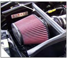
9. Press the weather seal onto the top of the Airaid Cool Air Dam. (<u>Hint</u>: begin at a corner and work the weather strip towards the ends)
