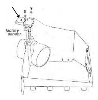
Fasten the factory sensor on top of the adapter using the (2) 8/32 screws and washers using a 3/32 Allen Wrench.
