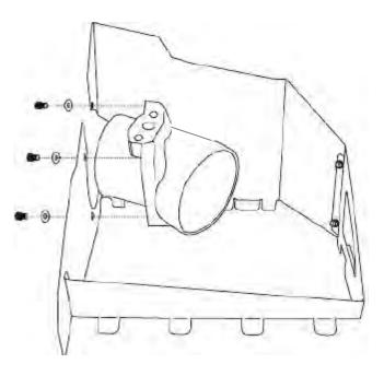
**4.** Assemble the air filter adapter to the cool air dam using the (3) <sup>1</sup>/<sub>4</sub>-20 bolts and washers provided.
