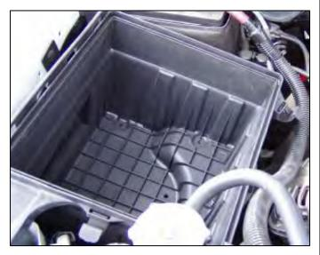
**2.** Unclip the factory air box lid and remove the lid assembly from vehicle.
