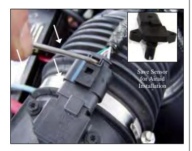
Disconnect the negative battery cable and disconnect the electrical connector. Using the T-20 bit loosen the two star head bolts and remove the electrical sensor. (Retain sensor for installation of Airaid Intake System)
