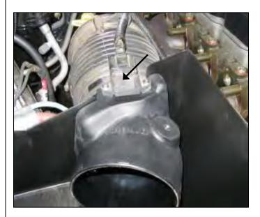
7. Re-connect the wire harness to the sensor on top of the Airaid adapter.
