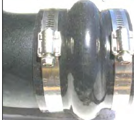
14. Install the urethane hump hose (#7) and urethane coupler (#8) onto the Airaid Intake Tube using four #60 hose clamps (#18). The coupler is positioned on the throttle body end and the hump hose is positioned on the air filter adapter end of the tube.
