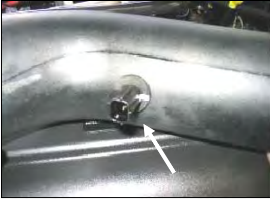
13. Install the rubber grommet (#17) and factory air temperature sensor into the Airaid Intake Tube (#6).
