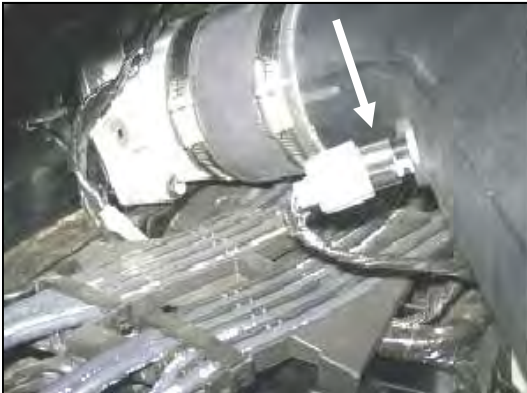
16. Reconnect the factory air temperature sensor wiring harness to the sensor. (It may be necessary on some late model vehicles to untape the wiring harness, extract approximately 2" of wire, and then retape the harness in order for the temperature sensor to be reconnected.)
