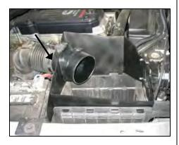
11. Install Airaid intake assembly in place of the factory air box lid & tighten factory hose clamp on intake tube to Airaid system & secure air intake tube to adapter using the factory hose clamp.
