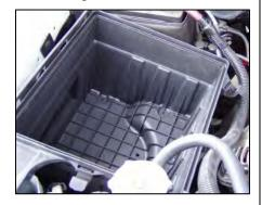
**3.** Unclip the factory air box lid and remove entire filter/intake assembly from vehicle.
