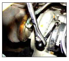
2. Loosen the hose clamp on the bottom of the factory intake tube that connects to the turbo housing.
