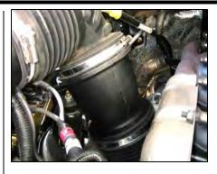
7. Check for any foreign objects or debris in the intake path & install complete tube assembly onto turbo charger using the stock hose clamp.
