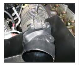
**12.** Re-connect the wire harness to the sensor on top of the Airaid adapter.
