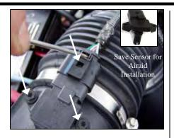
1. Disconnect the negative battery cable and disconnect the electrical connector. Using the T-20 bit loosen the two star head bolts and remove the electrical sensor. (Retain sensor for installation on Airaid Intake System)
