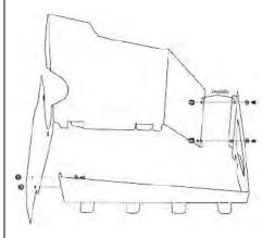
**8.** Assemble Airaid Quick Fit Cool Air Dam panels using the (4) 6/32 screws, washers and nuts provided.
