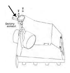
**10.** Fasten the factory sensor on top of the adapter using the (2) 8/32 screws and washers using a 3/32 Allen Wrench.
