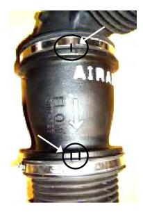
6. Note: on each side of the tube are notches that must be aligned with the notches on the stock connector tubes.
