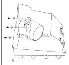
9. Assemble the air filter adapter to the cool air dam using the (3) \(^1/4\)-20 bolts and washers provided.
