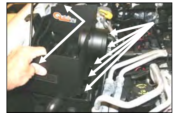
6. Slip the five tabs of the Quick fit panel (#2) through the slots on the airbox base. Adjust the panel for fit, then re-latch two of the factory clips onto the panel.
