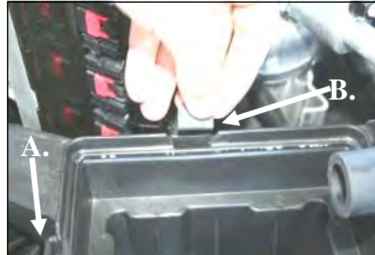
5. 2007 Models only: A.) Using a flat blade screwdriver, gently pry and remove one factory clip from the passenger side rear of the airbox base. (see arrow above) B.) Re-install the clip onto the rear of the factory airbox base (see arrow above).
