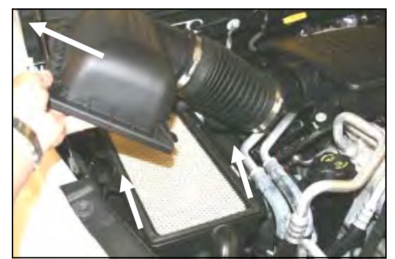
3. Remove the factory airbox lid and tube. Remove the factory air filter from the factory airbox base.
