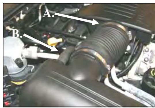
2. A.) Loosen the hose clamp on the resonator end of the intake tube. B.) Disconnect the breather hose from the factory airbox lid.
