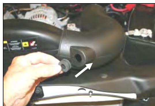
8. Install the grommet (#11) into the Airaid Intake Tube (#3).
