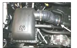
1. **Disconnect the negative battery cable!** Loosen the hose clamp on the resonator. Disconnect the breather hose going into the fac-
