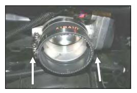
**10.** Install the reducing coupler (#5), small end first, onto the throttle body using two #52 hose clamps (#8). Leave the clamps loose for now.
