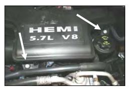
**4.** Using a 10mm socket, remove two bolts holding the intake resonator to the intake manifold. Lift and pull the resonator away from the throttle body and remove it from the vehicle.
