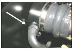
**15.** Slip the #24 speed clamp (#11) over the factory breather hose and re-connect the factory breather hose to the nipple on the Quick Fit Panel . Squeeze the clamp to retain the hose in place.
