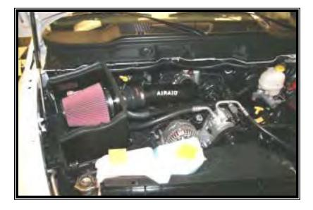
Synthamax Air Filters <u>do not</u> require <u>oil</u>. Service air filter as needed by cleaning with common non-petroleum all-purpose household cleaner and water. Simple Green®, Formula 409® or equivalent works great. Apply cleaner to outside of air filter and allow to soak. Then flush filter clean from the inside out with a garden hose and repeat steps if necessary. Do not apply
