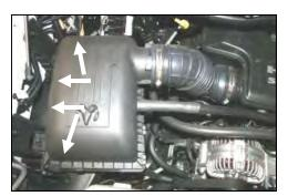
**2.** Unlatch 4 clips on the factory airbox lid and remove the lid and intake hose assembly. Remove the factory air filter.
