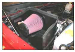
15. Install the Airaid Premium Filter (#1) onto the tube on the CAD and tighten the hose clamp. Next install the weather strip (#5) on the top of the CAD as shown. (Hint: Start at one corner and work towards the other corner. Don't start in the middle.)
