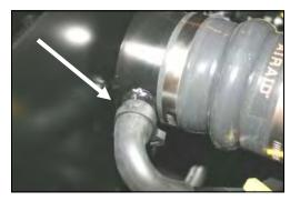
**12.** Install the provided #24 speed clamp (#9) over the factory breather hose, then slide the hose onto the nipple on the CAD. Squeeze the clamp to secure the hose.
