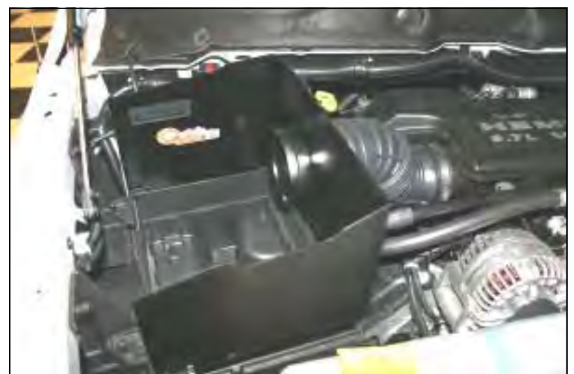
4. Install the Quick Fit Panel (#2) by slipping it into the factory intake tube, and then sliding it over the tabs on the factory airbox base. Adjust it for fit on top of the airbox base, and re-latch the 4 clips to hold the Quick Fit Panel securely in place.
