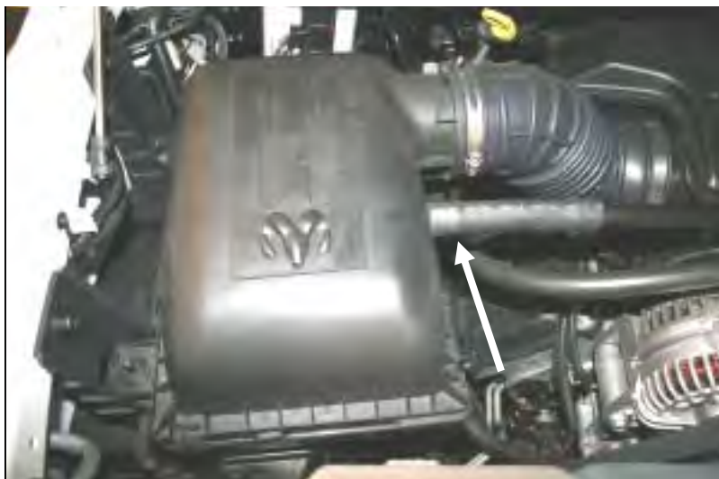
1. Disconnect the negative battery cable! Disconnect the factory breather hose from the air cleaner lid.
