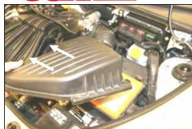
**3.** Remove the factory air cleaner lid by lifting up on the front, and then sliding the tabs out of the back of the air cleaner base.
