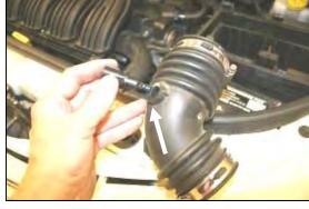
**6.** Carefully remove the temperature sensor from the factory intake tube and set it aside, it will be reused in step #10.
