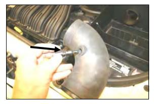
**10.** Very carefully, install the factory temperature sensor removed in step #6, into the Airaid intake tube. Make sure it is seated all the way in.
