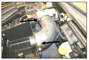
11. Install two #48 hose clamps (#7) on the Airaid intake tube, and then install the Airaid intake tube from the Quick Fit panel to the throttle body, making sure the reducer end is towards the throttle body. Tighten the hose clamps, and re-connect the temperature sensor wiring harness.
