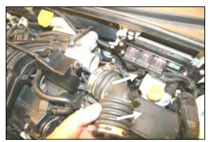
**5.** Remove the factory air intake tube from the throttle body.
