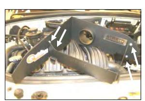
**7.** Assemble the Quick Fit Panels (#2 & #3) as shown, using the four provided screws (#8), washers (#9), and nuts (#10).
