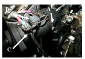
13. A) Slide the rubber elbow over the Airaid filter adapter, install one #80 hose clamp (#20), and tighten the hose clamp. B) Using three 8-32x1/2" button head screws (#13), reinstall the factory Mass Air Flow sensor, and temperature sensor into the Airaid filter adapter. Do Not Use The Factory Screws! C) Reinstall the wiring harness anchor into the hole in the filter adapter just below the temperature sensor.
