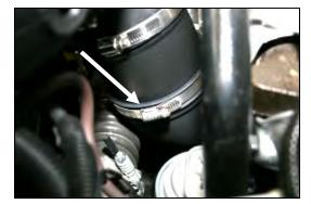
14. Tighten the factory hose clamp where the Airaid metal tube slips into the factory rubber elbow on the turbocharger.
