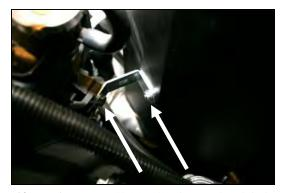
12. Using one 1/4-20x1/2" button head bolt (#11), 1/4" flat washer (#12), and 1/4" serrated nut (#13), and the 8x1.25x30mm hex bolt (#14), and 5/16" flat washer (#15), mount the supplied bracket (#19) between the CAD panel, and the fan shroud mounting boss as shown. Tighten all CAD mounting bolts at this time.
