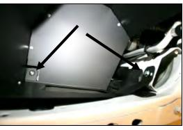
11. Install the CAD assembly into the vehicle, and install the 3/8-16x1" button head bolt (#18) thru the panel, and into the well nut. Next install the 6x1x12mm hex bolt (#16), and 1/4" flat washer (#12), thru the panel, and into the captured nut in the radiator support. Leave all bolts loose until final adjustment.
