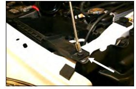
**3.** Using a 10mm socket, remove the nut that holds the front of the airbox base and grommet assembly to the radiator support.
