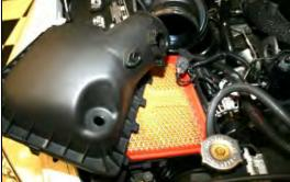
2. Unsnap the two metal clips that hold the airbox lid to the base, and remove the lid. Next, remove the factory paper air filter from the base.
