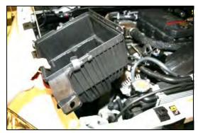
4. Gently rock the airbox base back and forth while pulling up, to remove it from it's mounting grommets, and remove it from the vehicle.
