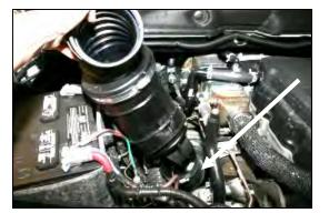
5. Loosen the factory hose clamp at the base of the factory plastic intake tube assembly, and remove the tube from the vehicle.
