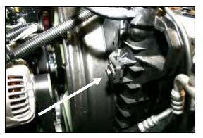
6. Using a 13mm socket, remove the factory bolt that holds the fan shroud to the radiator.
