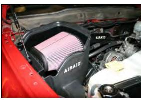
**14.** Install the Airaid Premium Filter (#1) onto the tube on the filter adapter and tighten the clamp. Next install the weather strip (#7) on the top of the Quick Fit Panel as shown. (*Hint: Start at one end of the* **CAD** *and work your way towards the other and*)
