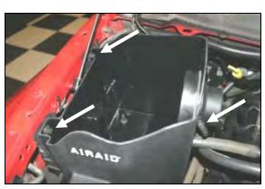
**9.** Install the **CAD** into the vehicle by aligning the grommets over the locating pins on the factory airbox mount. Reinstall the factory bolts in the fender that were removed in step #4. Next install the 1/4"NPT x 1/2" barbed fitting (#19) into the **CAD**.
