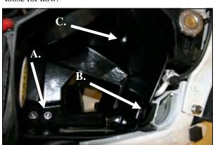
9. Install the CAB into the vehicle as shown. A.) Install the 3/8" button head bolt (#17) and flat washer (#18) thru the CAB and into the well nut. B.) Install the M6 x 25mm hex bolt (#15) and flat washer (#10) thru the CAB and into the captured nut in the fender. C.) Install the 5/16" bolt (#11) flat washer (#12), and flange nut (#13) thru the CAB and L-bracket. Tighten all mounting bolts at this time.
