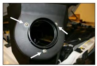
**8.** Install the filter adapter (#4) into the Cool Air Box (#3) using three 1/4" Button Head bolts (#9) and flat washers (#10) as shown.
