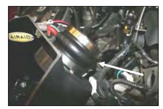
**10.** Install the supplied hump hose (#5) onto the filter adapter using two #72 hose clamps (#19). Leave the clamps loose for now.
