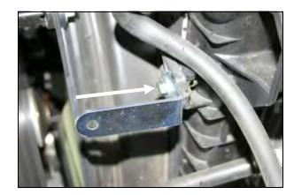
**6.** Install the L-bracket (#20) onto the radiator shroud as shown using one M8 x 30mm bolt (#14) and one flat washer (#12) as shown. Leave the bolt slightly loose for now.
