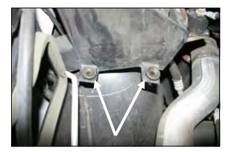
**4.** Remove the two grommets that held the factory airbox in position.
