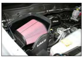
13. Slide the Airaid intake tube into the hump
