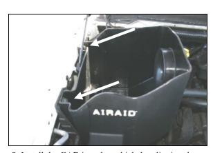
**8.** Install the **CAB** into the vehicle by aligning the grommets over the locating pins on the factory airbox mount. Reinstall the factory bolts thru the **CAB** and into the fender that were removed in step #4.
