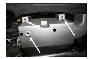
**6.** Install the three grommets removed in step #5 into the bottom of the Airaid Cool Air Box (CAB) (#2) at the locations shown here.
