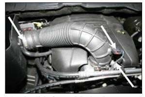
**13.** Reinstall the factory air intake tube. Reconnect the electrical connector to the temperature sensor, and then tighten both hose clamps.
