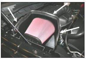
14. Install the Airaid Premium Filter (#1) onto the filter adapter and tighten the clamp. Next install the weather strip (#5) on the top of the CAB as shown. (Hint: Start at one end of the CAB and work your way towards the other end.)
