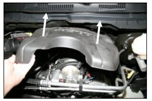
**2.** Lift up the front of the engine beauty cover, and then pull it towards you to remove it from the vehicle. It is only held in position by rubber grommets.
