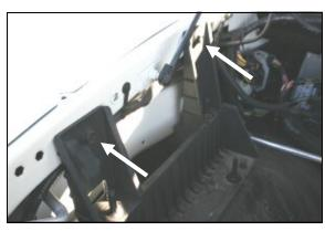
**5.** Using a 13mm socket, remove the two bolts that hold the airbox mount to the inside right fender. Save them for reinstallation in step #8.
