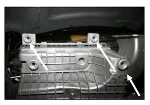
**5.** Remove and save three grommets from the bottom of the factory airbox. They will be reused in step #6.
