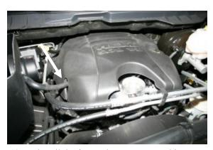
12. Reinstall the factory beauty cover making sure that the grommets are aligned with the grommet posts and that the crankcase breather hose is aligned in the slot on the side of the cover.
