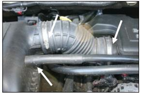
1. **Disconnect the negative battery cable!** Loosen the two hose clamps on the flexible intake tube, one at the airbox lid and one at the resonator. Slide the flexible tube off of the lid and the resonator and remove it from the vehicle.
