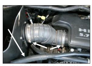
**9.** Reinstall the factory air intake tube and tighten the two hose clamps. Remove the rubber hose from the end of the factory crankcase breather tube.
