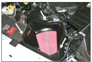
12. Install the Airaid Premium Filter (#1) onto the filter adapter and tighten the clamp. Install the weather strip onto the top of the **CAB** starting at the right fender and working your way towards the radiator.
