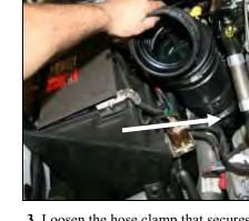
**3.** Loosen the hose clamp that secures the factory intake tube assembly to the rubber elbow on the turbo inlet, and remove the assembly from the vehicle..
