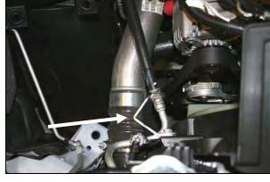
**6.** Install the bracket (#18) onto the radiator shroud as shown using the factory hardware. Leave the bolt slightly loose for now.
