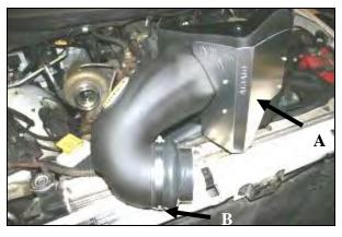
**5. A**) Install the aluminum Heat Shield (#4) onto the **CAB** using the four 1/4" Button head Bolts (#7) and the Flat washers (#8). Remove the protective film from Heat Shield. **B**) Install the silicone reducer (#5) on to the Airaid Intake Tube (#2) using the #80 (#14) Hose Clamp.
