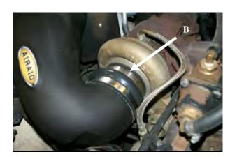
**7. A**) Install the **CAB** and Tube assembly onto the turbo inlet first, then rotate the assembly downward onto the inner fender studs. **B**) Secure the Silicone reducer to the turbo inlet using the # 64 Clamp (#13). **C**) Fully tighten the three 1/4" Button Head Bolts from step **4**.
