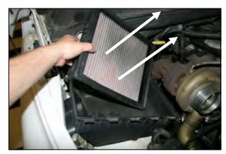
**2.** Remove the factory air filter from the lower half of the factory airbox.
