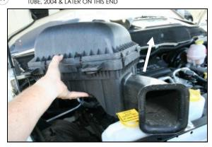
2. Rock the airbox back and forth as you are lifting it straight up to remove it from the vehicle. It is only held in by grommets.
