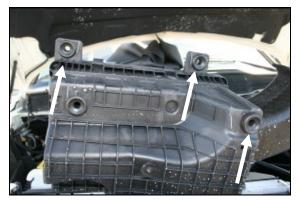
3. Remove and save three grommets from the bottom of the factory airbox. They will be reused in step #4.
