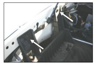
5. Using a 13mm socket, remove the two bolts that hold the airbox mount to the inside right fender. Save them for reinstallation in step #8.
