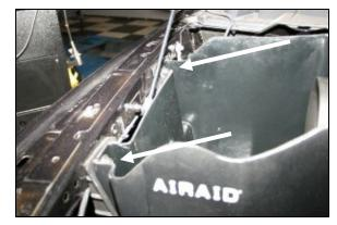
**9.** Install the **CAB** into the vehicle by aligning the grommets over the locating pins on the factory airbox mount. Reinstall the factory bolts into the fender that were removed in step #3.
