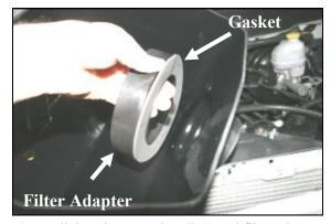
6. Install the adapter gasket (#12) and filter adapter (#3) into the CAB using three 1/4-20 x 5/8" bolts (#5) and flat washers (#6) as shown. Refer to the line drawing above for reference.
