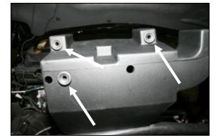
**6.** Install the three grommets removed in step #5 into the bottom of the Airaid Cool Air Box (CAB) (#2) at the locations shown here.
