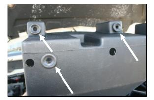
**4.** Install the three grommets removed in step # 3 into the bottom of the Airaid Cool Air Box (CAB) (#2) at the locations shown here.
