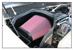
**11.** Install the Airaid Premium Filter (#1) onto the filter adapter and tighten the clamp. Next install the weather strip (#4) on the top of the **CAB** as shown. (*Hint: Start at one end of the* **CAB** *and work your way towards the other end.*)
