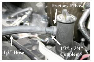
**10.** Install the supplied 1/2" x 3/4" plastic reducing coupler (#10), into the factory rubber elbow next to the oil fill neck as shown, and then connect the supplied 1/2" x 22" hose (#4) to the coupler.
