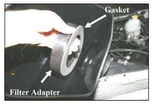
**7.** Install the adapter gasket (#12) and filter adapter (#3) into the **CAB** using three 1/4-20 x 5/8" bolts (#6) and flat washers (#7) as shown. *Refer to the line drawing above for reference.*
