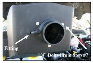
7. Install the 1/4" NPT x 1/2" barbed fitting (#8) into the filter adapter as shown. 2003 Models: Install the 1/4"NPT plug (#10) in place of the barbed fitting.
