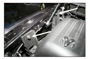
**3.** Using a 13mm socket, remove the two bolts that hold the air cleaner mount to the inside right fender. Save them for reinstallation in step #9.
