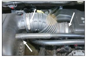
1. Disconnect the negative battery cable! Loosen the two hose clamps on the flexible intake tube, one at the airbox lid and one at the resonator. Slide the flexible tube off of the lid and the resonator and remove it from the vehicle. 2004-08 Models: Disconnect the crankcase breather hose that attaches to the factory airbox lid.
