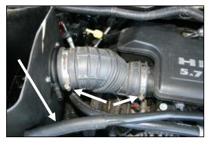
9. Reinstall the factory air intake tube and tighten the two hose clamps. Remove the rubber hose from the end of the factory crankcase breather tube.
