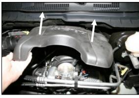
**2.** Lift up the front of the engine beauty cover, and then pull it towards you to remove it from the vehicle. It is only held in position by rubber grommets.
