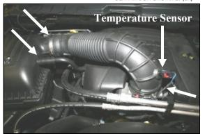
1. **Disconnect the negative battery cable! 2009 Models:** Locate the temperature sensor on the air intake tube, slide the red tab, squeeze the black tab on the electrical connector, and then disconnect the temperature sensor from the air intake tube. Disconnect the crankcase breather tube from the air filter box. Loosen one hose clamp at each end of the air intake tube and remove it from the vehicle.
