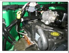
4. Remove air filter assembly from engine compartment. Retain rubber throttle body coupler for later use.
