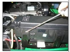
5. Using a flat blade screwdriver, unclip the fuse box from the bracket and set aside. Using 10mm socket, remove bolt from bracket. (*Note: Retain bolt for later use.*)
