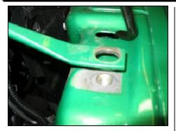
1. Disconnect the negative battery cable. Remove bolt for radiator support rod. (<u>Note</u>: *Retain bolt for later use.*)
