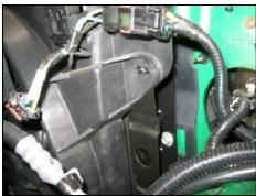
6. Using a 7/16" socket, remove the bolt located on the radiator fan cover on the passenger side. (<u>Note</u>: Retain bolt for later use.)
