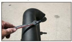
**14.** Install the <sup>1</sup>/<sub>4</sub>" barbed fitting into the intake tube.
