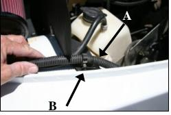
**12.** A) Using a <sup>1</sup>/4"x20 bolt, washers, and nut, bolt the CAD to the fender. B) Install the wire loom clamp into the hole in the CAD, as shown.
