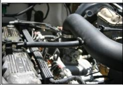
**17.** Replace the factory breather hose with ½"x10" rubber hose between valve cover and intake tube using speed clamps as shown.
