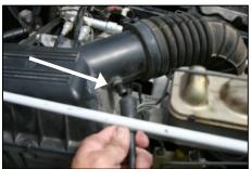
2. Unhook vacuum line from airbox, and remove from vehicle at the canister below the master cylinder. (Save for later use.)
