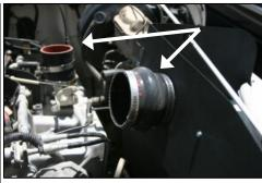
**15.** Install hump hose on CAD with #52 hose clamps, and the coupler on the throttle body with #44 hose clamps as shown.
