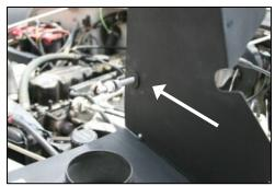
**9.** Carefully slide the CAD over the support rod, and then slide the supplied grommet over the rod, and into the hole in the CAD as shown. Rotate the CAD and place into position on the factory airbox mount. Reinstall the radiator support rod, and tighten the nut.
