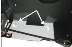
**10.** Install two ¼"x20 bolts and washers thru the top, and fender washers and nuts on the bottom, where the factory grommets were removed.
