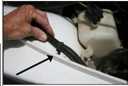
**6.** Carefully remove wire loom clamp from hole in fender.
