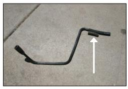
**13.** Remove the factory hose from step 2, and install the new 3/8"x4" hose on the end of the vacuum line as shown. Reinstall vacuum line. (Refer to step 2.)
