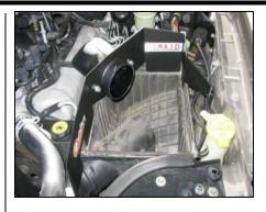
7. Position the Airaid Cool Air Dam in place of the factory air box and snap into place.
