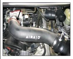
9. Position the Airaid Modular Intake Tube assembly to connect the reducer to the throttle body and the hump hose to the Airaid Cool Air Dam. (Note: leave the hose clamps loose until final assembly)
