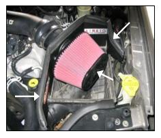
**11.** Mount the Airaid Premium filter & weather strip onto the Cool Air Dam. (*Hint*: start the weather strip at a corner and work towards the ends)
