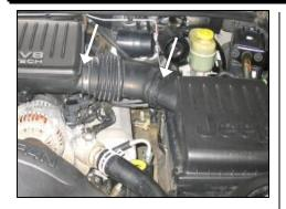
1. Disconnect the negative battery cable, and then loosen both of the hose clamps to factory tube connecting factory air filter assembly to factory air box silencer.
