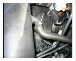
10. Connect the factory breather hose the Airaid Modular Intake Tube & secure hose with the #16 black speed clamp provided.
