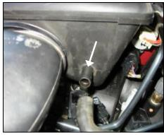
**3.** Disconnect the breather hose from the factory air box silencer.
