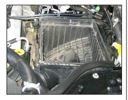
2. Remove the factory air filter box lid, accordion tube, and air filter. (Note: leave factory air filter base installed in vehicle)
