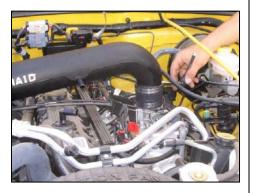
**22.** Install Airaid intake tube by connecting both ends into the rubber hump hose and reducer.
