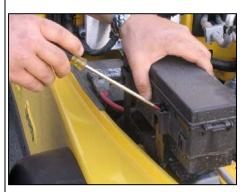
7. Using a flat blade screwdriver, push locking tabs inward to remove the fuse panel from the mounting bracket. Position panel out of the way to access the bolt underneath.
