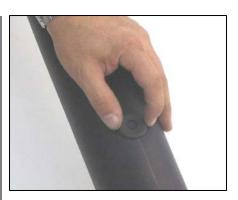
**17.** For 1997-2004 vehicles only: Install the supplied rubber grommet with out the hole into the Airaid intake tube.
