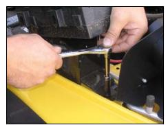
**13.** Align the mounting holes in the Airaid Cool Air Dam with the factory holes in the inner fender. Using the original bolts from step 7, mount the Airaid Cool Air Dam to the inner fender.
