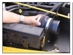
**20.** Install rubber hump hose and two #64 hose clamps on end of the Airaid Cool Air Dam. Leave hose clamps loose until final assembly.
