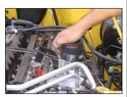
**21.** Install rubber reducer on throttle body with two #44 hose clamps. Leave hose clamps loose until final assembly.
