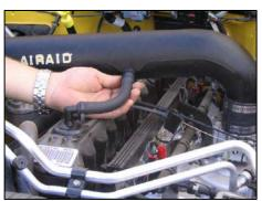
24. Connect the other end of the valve cover hose to the intake tube. Secure both ends of the hose using the supplied black speed clamps.
