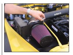
**26.** Install the Airaid Premium Filter on the Cool Air Dam assembly. Secure the filter using the supplied hose clamp.
