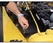
14. Using the supplied ¼ x 20 nut, bolt and washers, mount the front of the Airaid Cool Air Dam to the inner fender.
