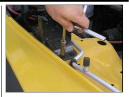
8. Using a 10mm socket, remove one bolt from the inner fender as shown above. Retain bolt for later use.
