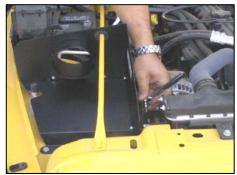
**15.** Using the original bolt from step 5, mount the Airaid Cool Air Dam to the passenger side radiator mount.
