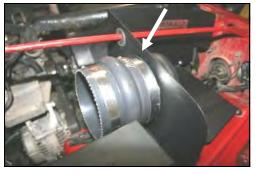
**16.** Install the urethane hump hose (#5) onto the back side of the **CAD** tube using two #72 hose clamps (#17). Tighten <u>only</u> the hose clamp on the metal tube for now.
