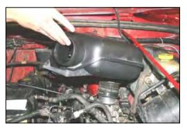
**6.** Remove the resonator from the vehicle.
