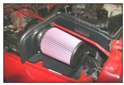
**22.** Install the Airaid Premium Filter (#1) onto the **CAD** tube and tighten the hose clamp. Next, install the weather strip (#7) onto the top of the CAD as shown, starting at the fender, working your way towards the radiator.
