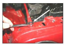
10. Remove and save the bolt from the passenger side radiator support brace. It will be re-used in step #13.
