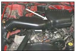
Disconnect the negative battery cable. Loosen the hose clamp that holds the factory intake tube to the resonator.
