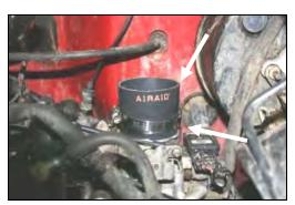
**17.** Install the reducer (#6) onto the throttle body using two #44 hose clamps (#16). Tighten only the hose clamp on the throttle body for now..
