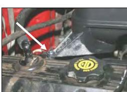
**5.** Remove the bolt that holds the resonator to the valve cover.
