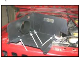
11. Assemble the two Cool Air Dam panels (#2) & (#3) using the four 6-32 screws (#8), #6 flat washers (#9), and nuts (#10), as shown.
