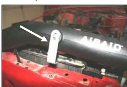
**18.** Install the L-bracket (#18), onto the Airaid Intake Tube (#4), using one 1/4" button head bolt (#11), and flat washer (#12). Leave the bolt loose for now.
