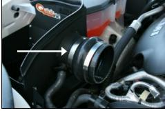
**14.** Install the hump hose and two #56 hose clamps on the Quick Fit assembly. **Do not tighten** the clamps at this time.
