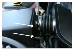
Disconnect the negative battery cable. Loosen the hose clamp on air cleaner box lid. Twist and remove breather hose from air cleaner box lid.
