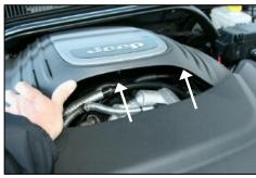
**6.** Carefully lift up on the engine cover (*it is held in place by grommets, no bolts*) to access the hose clamp on the throttle body, and 10mm bolt next to the throttle body.
