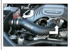
18. Carefully install the end of the tube into the hump hose, and then into the coupler on the throttle body as shown. Adjust the tube as needed, and tighten the four hose clamps.
