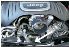
15. Install the coupler and two #56 hose clamps on the throttle body as shown. Do not tighten the clamps at this time. Secure the breather hose to the air conditioner line using the supplied zip tie.
