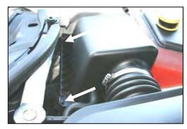
**2.** Unhook the two air cleaner lid latches on the front of the airbox.
