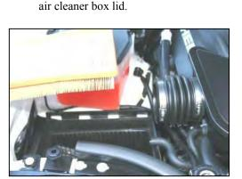
**4.** Remove factory air filter from the air cleaner box.
