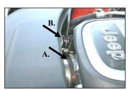
7. A.) Loosen the hose clamp on the throttle body. B.) With a 10mm socket, remove the bolt next to the throttle body that holds the intake resonator in place.
