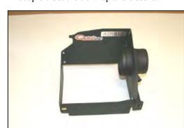
11. Assemble the two pieces of the Quick Fit panels as shown (#2&#3), using the four 6-32 screws (#12), washers (#13), and nuts (#14), that are provided in the kit.
