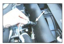
**17.** Carefully install the factory temperature sensor into the grommet. Make sure it is seated all the way in.
