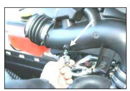
**10.** Carefully twist and remove the temperature sensor from the bottom of the resonator, and then remove the resonator from the vehicle.
