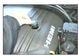
5. Remove, and set aside the oil filler cap.
