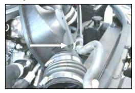
**9.** Slide the clip off of the resonator that holds the breather tube in place.
