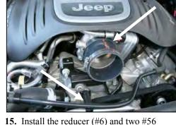
15. Install the reducer (#6) and two #56 hose clamps (#9) on the throttle body as shown. **Do not tighten** the clamps at this time. Secure the breather hose to the air conditioner line using the supplied zip tie (#15).
