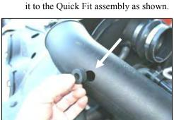
**16.** Install the supplied grommet (#8) into the hole in the back of the tube.
