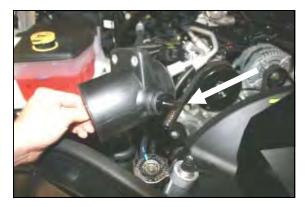
**10.** Install the supplied 90° nylon fitting (#9), into the air filter adapter (#4) as shown.
