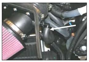
**18.** Reconnect the factory breather hose onto the 90° nylon fitting (#9).
