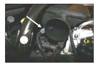
6. Disconnect the intake air temperature sensor wiring harness, by squeezing the tab on the side, and
