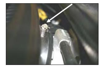
7. Using a 5/16" socket, ratchet and extension (or flat blade screw driver), loosen the hose clamp on the throttle body. This clamp is located close to the firewall, in the center of the engine compartment.
