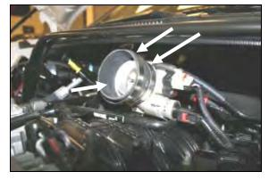
**12.** Install the provided reducer (#6) onto the throttle body with the smaller diameter towards the throttle body. Place the #48 hose clamp (#13) on the smaller diameter section of the reducer (throttle body side). Place the #52 hose clamp (#14) on the larger diameter side of the reducer. Leave the clamps loose for now.
