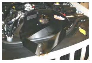
9. Assemble the Quick Fit panels (#2, #3) as shown, using five 6-32 screws (#16), #6 flat washers (#17), and 6-32 keps nuts (#18).
