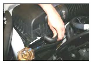
3. Disconnect the factory breather tube from the air cleaner box lid.
