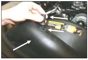
**15.** Install the rubber grommet (#12) into the Modular Intake Tube (#5). Next, slide the factory intake air temperature sensor into the grommet in the tube. Make sure it is seated all of the way in.
