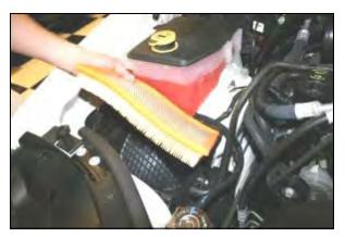
5. Remove the factory air filter.
