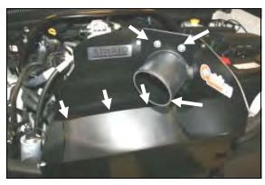
**11.** Install the Quick Fit panels into the factory lower airbox by lining up the three tabs in the rear of the panel, and the latch holes in the front, and then re-latching the factory airbox clips. Next, using two  $1/4-20 \times 1/2$ " button head screws (#10) and 1/4" flat washers (#11), install the air filter adapter into the Quick Fit Panel.
