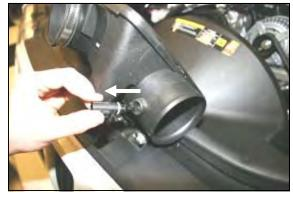
**14.** Remove the factory intake air temperature sensor from the resonator box by carefully twisting the sensor body, and pulling it straight out of its mount. Place the sensor in a safe location, it will be re-used in step #15.
