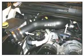
**16.** A.) Install the Modular Intake tube into the hump hose end first. B.) Insert the opposite end of the Modular Intake tube into the reducer, on the throttle body. Adjust the components for fit, and then tighten all of the hose clamps, and reconnect the factory intake air temp sensor wiring harness.
