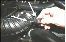
1. **Disconnect the negative battery cable.** Disconnect the wiring harness connected to the air temperature sensor. <u>WARNING!</u> Electrical connector & sensor are very fragile. <u>USE CAUTION !</u> <u>Very Carefully</u> remove the temperature sensor from the factory intake tube by using a small circular motion while pulling it straight out.
