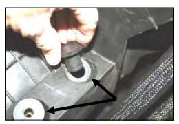
**7.** Using a 10mm socket, remove and save the bolt from the factory plastic air cleaner mount. It will be re-installed in step #12.
