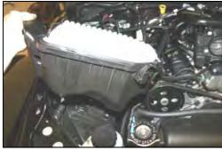
**5.** While rocking the factory air cleaner base back and forth, pull up, and remove it from the vehicle. There are no bolts holding it down, just grommets.
