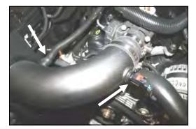
17. Very Carefully reinstall the temperature sensor removed in step #1, into the grommet in the Airaid Intake Tube, and then reconnect the wiring harness. Reconnect the factory breather hose to the nipple on the intake tube, and install the supplied speed clamp (#19) over the hose.
