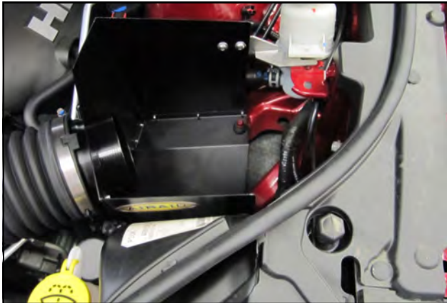
13. Install the Panel assembly into the engine compartment as shown. Slide the Mounting bracket underneath the power steering reservoir and the airbox mounting post through the grommet in the Panel. Secure the assembly by reusing the bolt from step 12. Connect the factory intake tube to the Airaid Intake tube and tighten the clamp.
