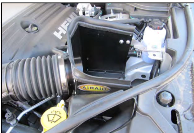
16. Install the Weather Strip (#4) to the top edge of the panels, and reattach the hood seal.
