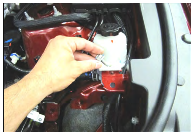
12. Remove the bolt securing the power steering reservoir and set it aside. This bolt will be reused in step 13. to hold the Mounting bracket.
