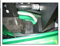
9. Reinstall original bolt through Airaid Cool Air Dam and factory fuse block bracket. Replace fuse block on bracket.
