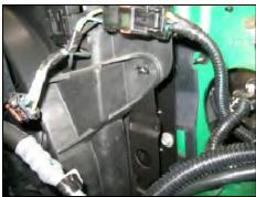
6. Using a 7/16" socket, remove the bolt located on the radiator fan cover on the passenger side. (*Note*: *Retain bolt for later use.*)
