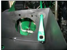
8. Position Airaid Cool Air Dam in place by inserting factory radiator support rod through grommet as shown.
