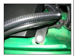
**11.** Using the supplied hardware and 7/16" socket, fasten the front of the Airaid Cool Air Dam to the fender.
