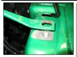
1. Disconnect the negative battery cable. Remove bolt for radiator support rod. (*Note: Retain bolt for later use.*)
