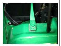
**12.** Using a <sup>1</sup>/<sub>2</sub>" socket, reinstall the original bolt on the radiator support rod.
