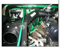
13. Install factory throttle body coupler on end of Airaid intake tube and position assembly on engine as shown. Mount Airaid intake tube to Cool Air Dam using two supplied ¼"-20 bolts and washers provided. Connect factory breather hose to Airaid intake tube.
