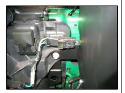
**10.** Using a 7/16" socket, reinstall the original bolt through the Airaid Cool Air Dam and radiator fan cover.
